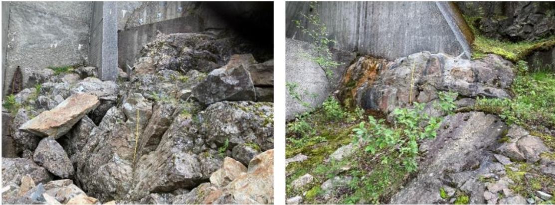
Figure v7: Left: Heavily fractured granitic gneiss at bottom of southern valley side, near support F. Right: massive granitic gneiss near top of southern valley side, between support H-I.
