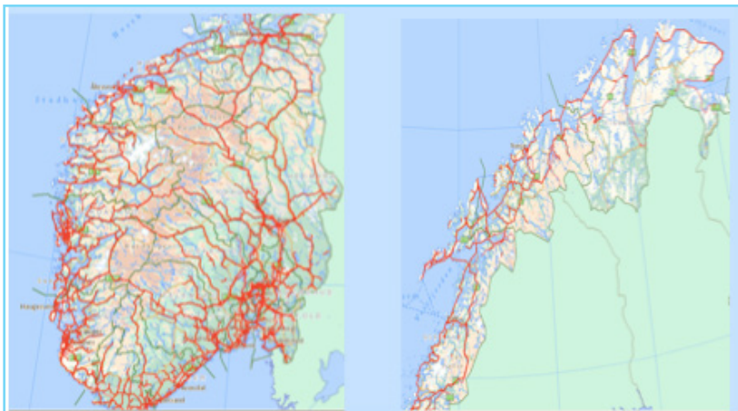
FIGURE 9-1 Telenor fiber grid in Norway.
