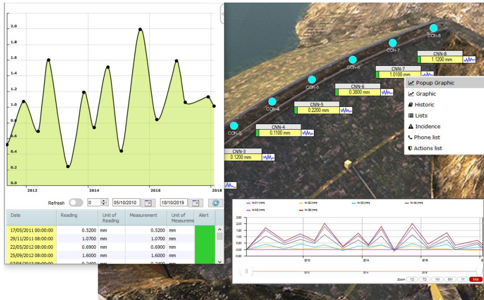
Figure 30: Visualization of a 3D dam view in combination with tooltips and popup charts.
