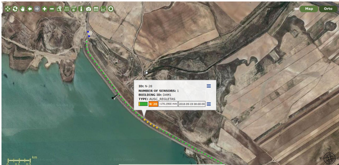
Figure 32: Location of monitoring pegs on a dam crest showing alarm levels.
