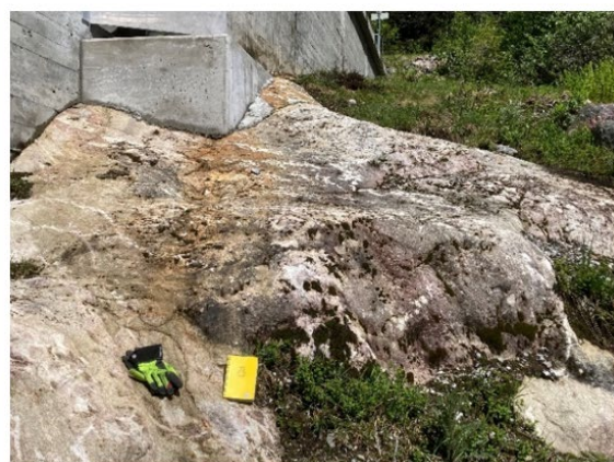
Figure 103. Dam 2: Very massive amphibolite between P7-Ø1 (left) and migmatite at N-end (right).
