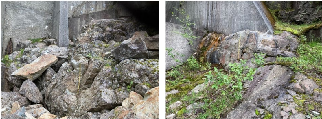
Figure 69: Left: Heavily fractured granitic gneiss at bottom of southern valley side, near support F. Right: massive granitic gneiss near top of southern valley side, between support H-I.
